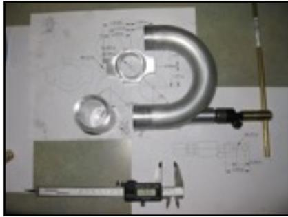
*Top: Layout and prototypes parts of an aluminum manifold*
